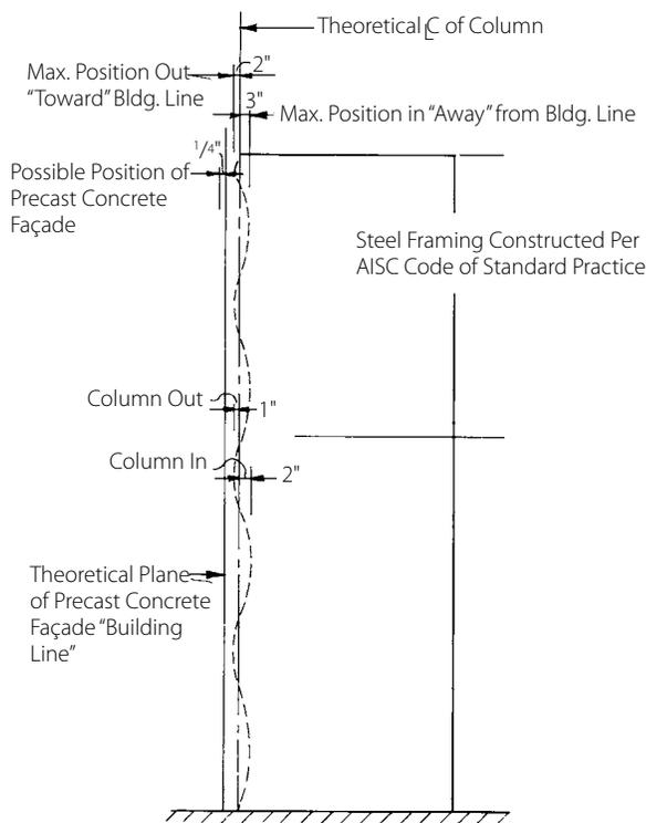
**Figure 4** Clearance example. Note: 1 in. = 25.4 mm.
