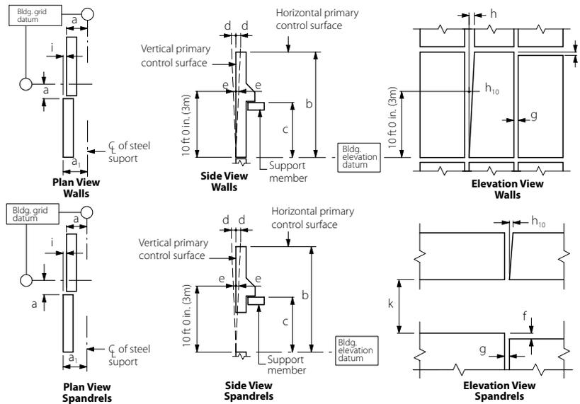
The primary control surfaces are usually as shown, although this needs to be confirmed on a job-by-job basis.
