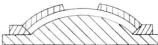
G: & H: EXTREME RADIUS More complex formwork with sequential back pans that must be removed and replaced daily. Also, casting time takes longer and some back finishing is required.
