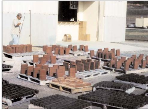
Before each individual brick is handset, a retarder is applied that facilitates cleaning of any mortar that might seep onto the face of the brick when the concrete face mix is poured. Rebar is then added, cost-saving "back-up" concrete is poured, and then the connection hardware is set.
