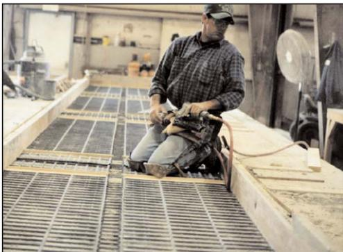
Building a mold is the first step in preparing to pour a brick-laid precast panel. Form liners which are produced to simulate a traditional laid brick pattern are placed in the bottom of the mold to act as a gasket for the brick when the concrete is poured.
